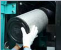
Double-element air cleaner The large-capacity element features a double-filter structure that keeps the engine running clean even in dusty environments.
