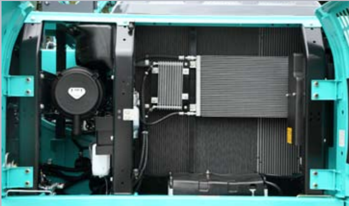
Double-element air cleaner The large-capacity element features a double-filter structure that keeps the engine running clean even in dusty environments.
